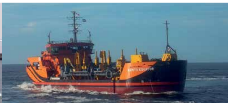
TSHD2500 FITTED OUT FOR MAINTENANCE DREDGING JOBS
