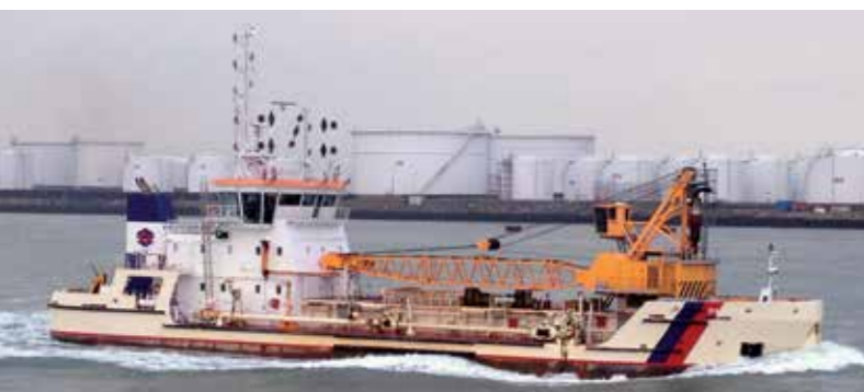
TSHD700 'GAMBE D'AMFARD' IS A FULLY CUSTOMISED DREDGER
