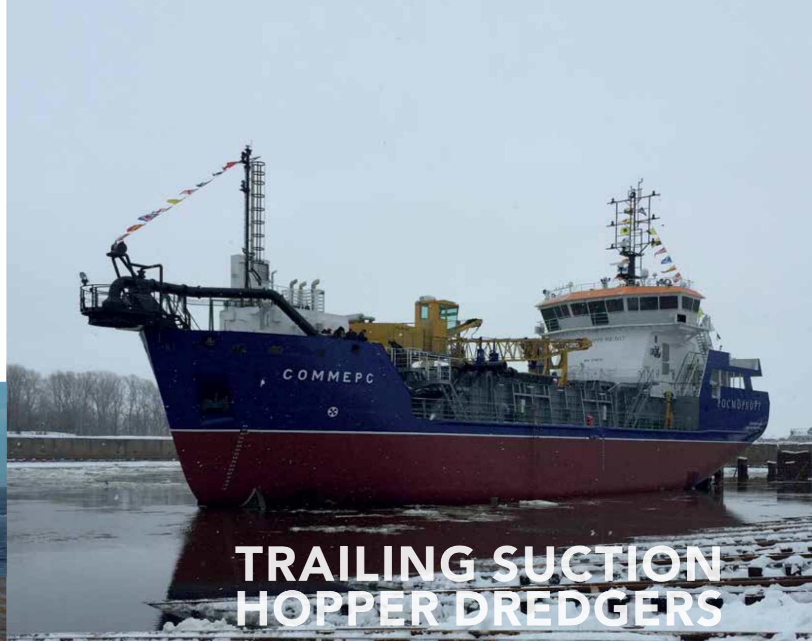
TSHD2500 FITTED OUT FOR MAINTENANCE DREDGING JOBS
