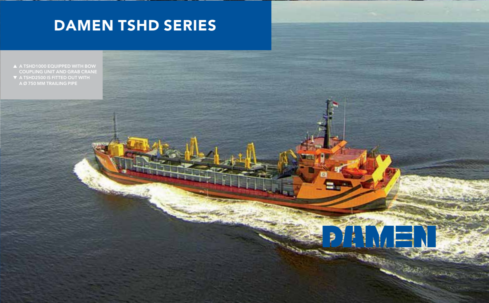
TSHD600 WITH A GRAB FITTED FOR DREDGING COMPACTED SEDIMENTS
